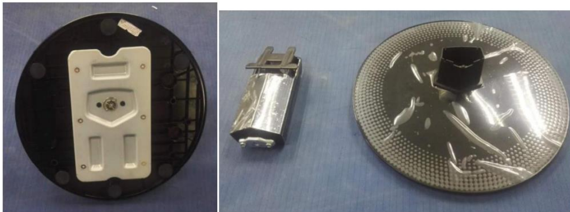
Step11. Unscrew two screws and separate base & neck assembly
